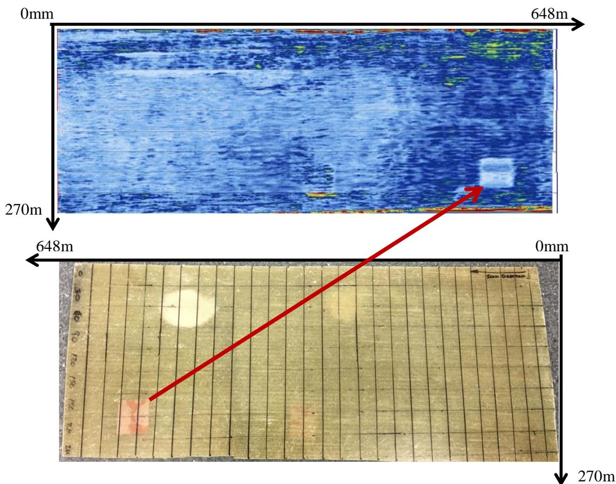
With the Autowinspec AU system, all three teflon inserts were detected:
